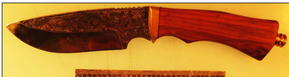
Fig. 1. Type of knife with a sharpening angle of 74^{\circ}
